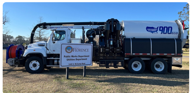
The City's new 900 Service Vector truck cleans and vacuums sanitary sewer and stormwater systems, removing grease, debris, and roots to maintain proper flow.
